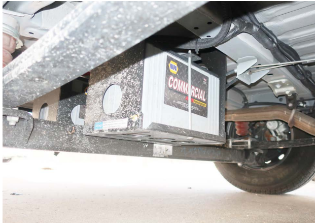
House Battery Access (Located behind rear tires) - Remove bolts from battery retainer to remove house battery
