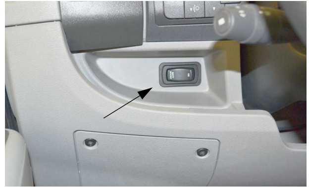
Battery Boost Switch
