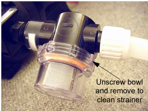
Water Pump Strainer -Typical View
