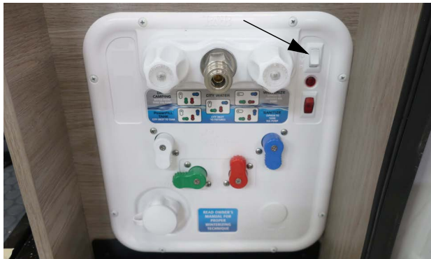
Pump switch -Typical View
